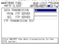
5. Use the **arrow keys** to select FTP TRANSMISSION TEST, and press **SELECT**. Press **SELECT** to transfer the file.
