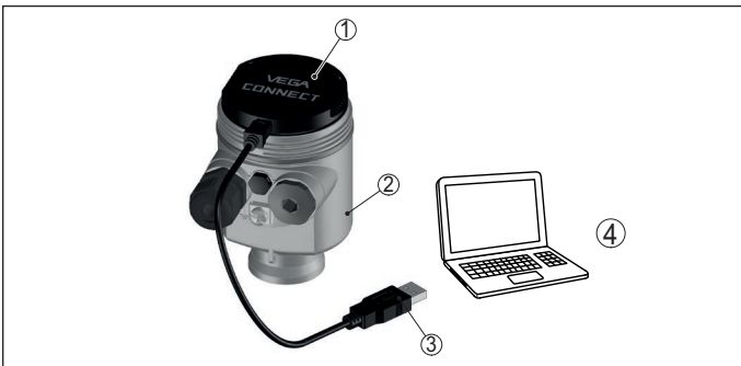
Fig. 20: Connection of the PC via VEGACONNECT and USB
