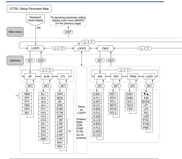
Pressing the DISP key once when a parameter setting display is shown retrieves the submenu of that parameter setting display.
