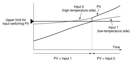
Switching at the Input Switching PV Upper Limit for PV Switching
