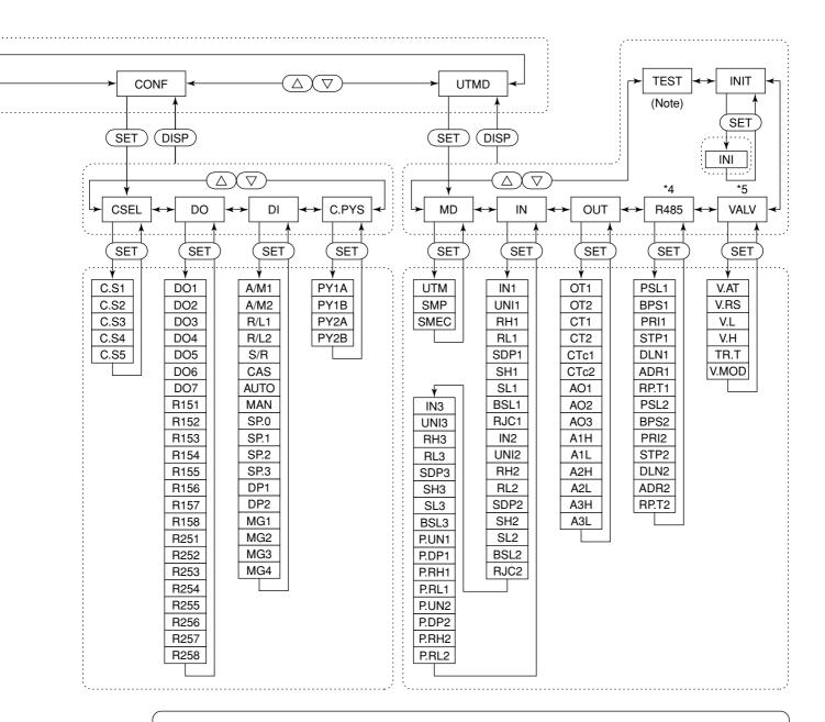
Note: The parameter items shown on the [TEST] submenu of the setup parameter setting display are to be used by Yokogawa service personnel to check the controller functions. User cannot set or change these parameters.
