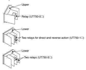
6. Pull out the relay to be replaced.
