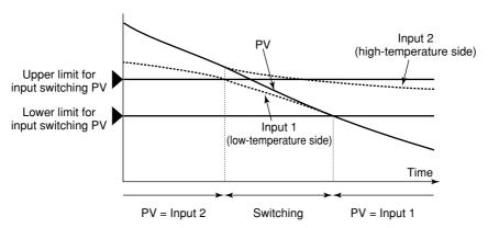
Switching within Specified PV Range (Falling PV)
