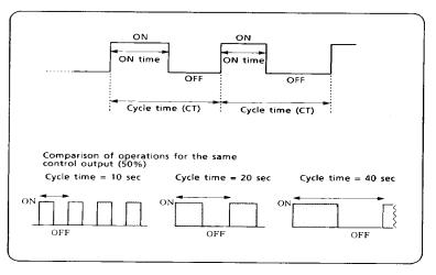
Control output pulse width = control output (%) x cycle time.
