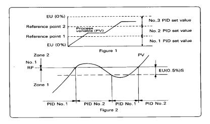
The 4<sup>th</sup> PID set is selected when the deviation from setpoint exceeds the value R.DV entered with PID4. This is shown below.
