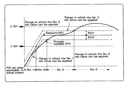
*Important Note:* During auto tune, when ZON is on, the auto tune will occur at the midpoint of the zone no matter what setpoint is selected.
