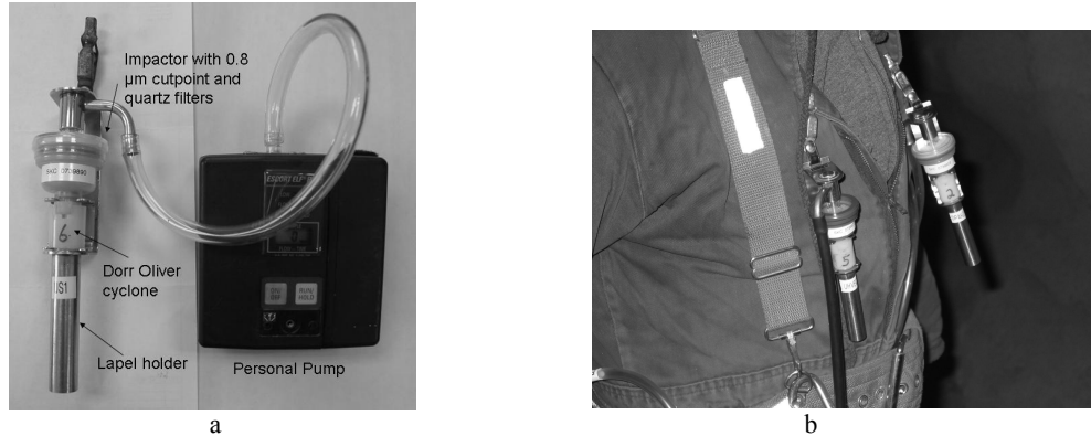
Figure 2: (a) The standard sampling setup which consists of an impactor with two quartz fiber filters inside attached to a cyclone in a lapel holder. Tubing connects the lapel holder to the personal pump. (b) The setup is designed to be worn by the miner by attaching the lapel holder to the clothing and the pump to the miner's belt.
