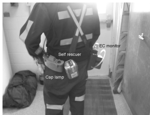
Figure 4: EC monitor is designed to be worn by a miner. It fits on the miner's belt with a camp lamp and self rescuer.
