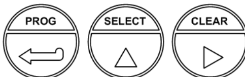
Fig. 2: Control panel, optical keys.
