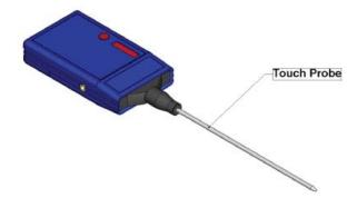
The patented Touch Probe accessory is a device that converts solid-borne sounds into airborne sound the Tru Pointe<sup>®</sup> Ultra can detect. For example, the sound of an internal leak in a water valve will travel to its surface. Touching the surface of the valve with the Touch Probe transfers the ultrasound into the probe and converts it to airborne ultrasound. To install the Touch Probe:
