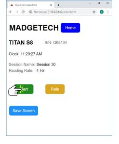
Home > Start Logging > Select New Reading Rate > Start > The reading rate was changed to 1 KHz from 4 Hz. Click the Start button to start data logging and return to the Home Screen.
