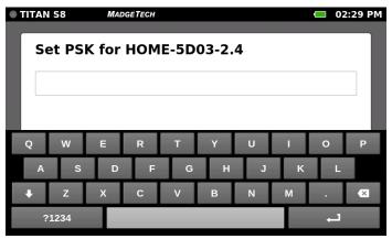
Enter the Wi-Fi SSID password which can be any character on the virtual keyboard displayed on the Titan S8 screen. Space and double quote characters are not permitted for the PSK.
