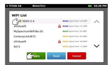
After scanning, the available SSID's are displayed. The red open lock means the Wi-Fi SSID is not secured with a password. The list is sorted by signal strength with the strongest signal at the top of the list. Any hidden SSID will not show up in this list.
