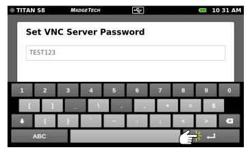
Press in the text box to bring up the virtual keyboard. Some keys are disabled as those characters are not permitted in the Password. Select the Up/Down (Shift) arrow to access additional special characters. The VNC Server Password must be over five characters. Select **Enter** key when finished entering the Password.
