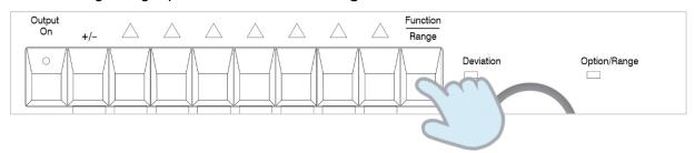
Now reselect the present function. For example, for DC volts, press the "**DC V**" button.
