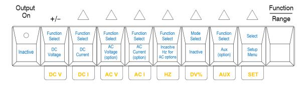
The **Function/Range** button can also be pressed after a function has been selected and is in use. The function indicators will flash show they are selectable. Any modes or setting buttons available for use will also flash. The user can choose to:
