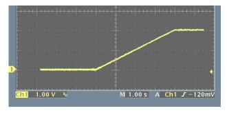
An oscilloscope trace showing a ramp from 0V to 2V in 4 seconds
