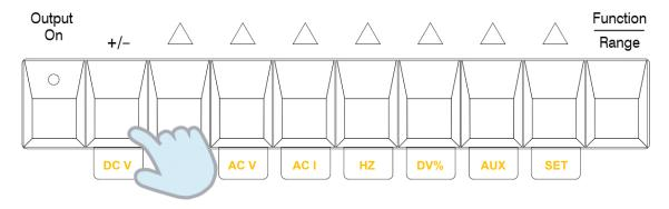
Once pressed, the function (DC V) will be the only indicator to remain illuminated, showing it is the selected function.
