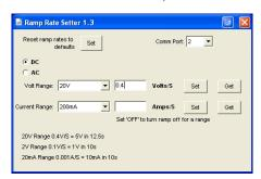
The ramp rate is held in non-volatile memory, so settings are retained even if the unit is switched off. Ramping is precisely controlled by the 5018's internal micro-processor and does not require connection to a PC to perform the actual ramping function.
