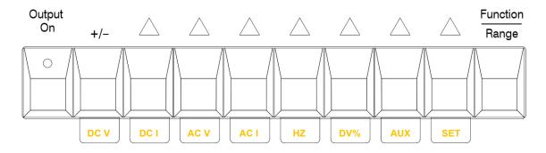
3. Select the desired function by pressing adjacent button. In this example DC Voltage.
