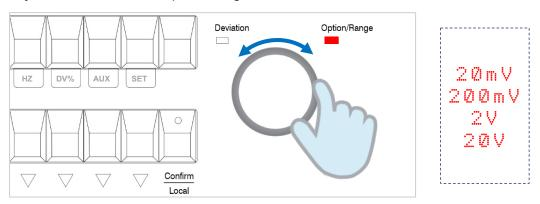
When the required range is displayed, press the "**Confirm**" button as highlighted by the flashing LED.
