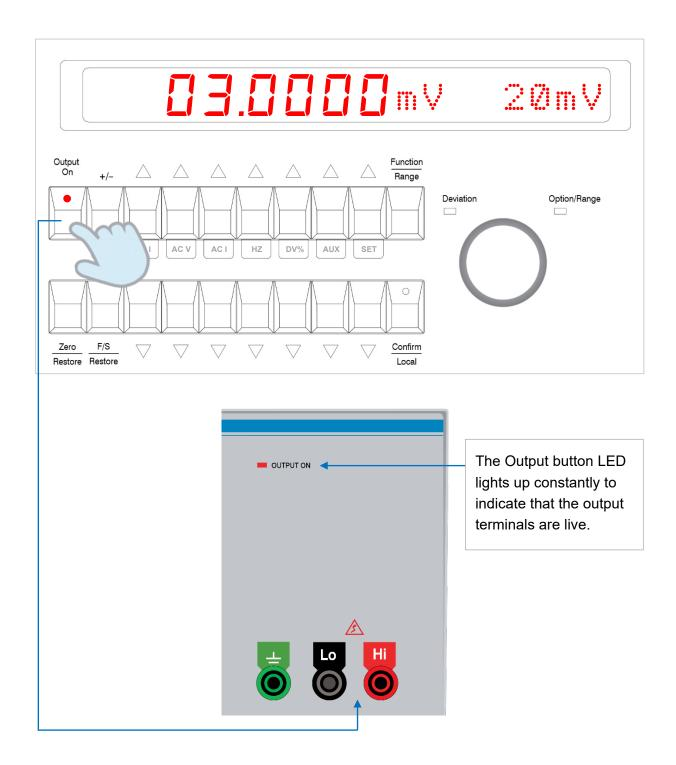
5. To change the output level, the **Up** ( $\Delta$ ) / **Down** ( $\nabla$ ) buttons can be used at any time.
