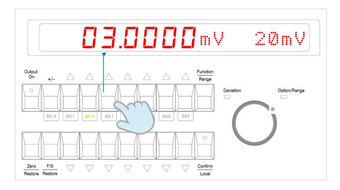
Output is initially disconnected from the output terminals. The LED on the Output On button flashes to indicate this. The LED beside the output terminals also flashes.
