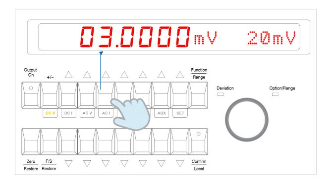
The polarity of the output can be changed by pressing the "+/-" button.
