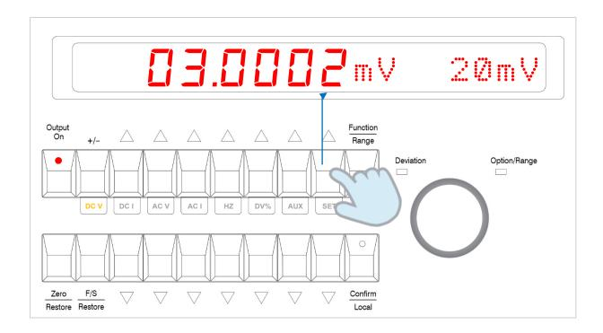
If necessary, the output can be turned off by pressing the "Output On" button.
