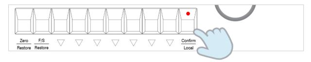
4. Once the frequency is set, the display readout will show the output voltage and operating range. The output value can be entered using the "**Up** ( $\Delta$ ) / **Down** ( $\nabla$ )" buttons.
