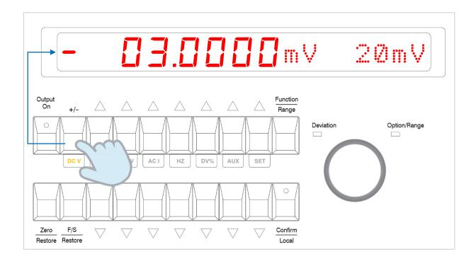
It is possible to set the output to zero in one step by pressing the "Zero" button.
