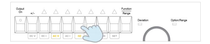
Select the frequency using the "Up ( $\Delta$ ) / Down ( $\nabla$ )" buttons.
