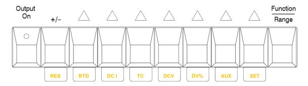
3. Select the desired function by pressing adjacent button. In this example **Resistance**.
