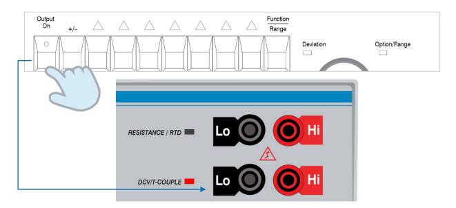
To change the units of temperature (Celsius, Fahrenheit or Kelvin), use the Setup menu. **Note:** Thermocouple outputs are cold junction compensated.
