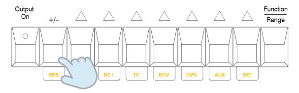
Once pressed, the function (RES) will be the only indicator to remain illuminated, showing it is the selected function.
