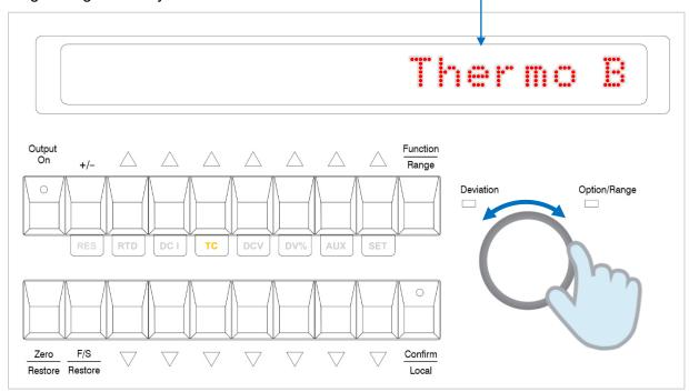
Press the "Confirm" button once the required thermocouple type is selected. Then set the required temperature value using the "Up ( $\Delta$ ) / Down ( $\nabla$ )" buttons. Deviation mode is available. To use press the "Function" button, then "DEV" button. Connect the output to the terminals by pressing the "Output On" button.
