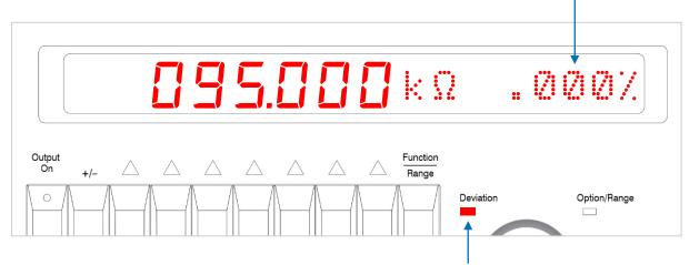
Deviation mode is highlighted by illumination of the "Deviation" LED. This prompts the use of the rotary knob.
