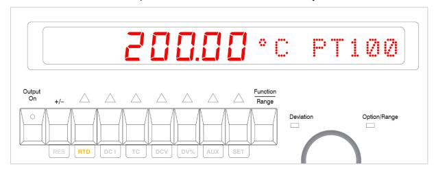
Then set the required temperature value using the "**Up** ( $\Delta$ ) / **Down** ( $\nabla$ )" buttons. Deviation mode is available. To use press the "**Function**" button, then "**DEV**" button. In deviation mode the PT100 indication is replaced by the % up/down setting.  $\neg$
