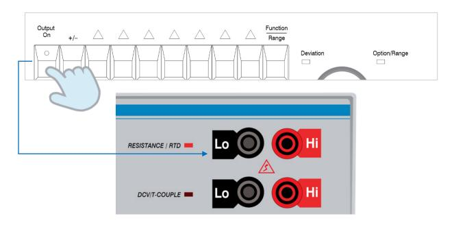
Note: External lead resistance must be subtracted from the final output value.
