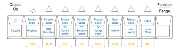
The **Function/Range** button can also be pressed after a function has been selected and is in use. The function indicators will flash show they are selectable. Any modes or setting buttons available for use will also flash. The user can choose to:
