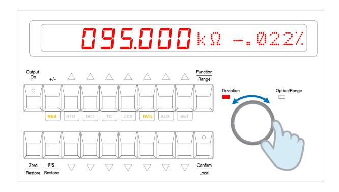
**Note:** It is not possible to adjust the deviation if the output setting is zero, since the deviation is a percentage of value. The deviation will be displayed as zero percent in this case.
