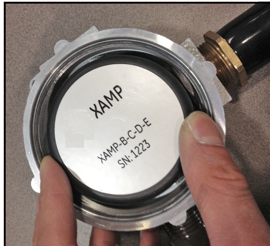
Figure 22: Junction Box Cap
