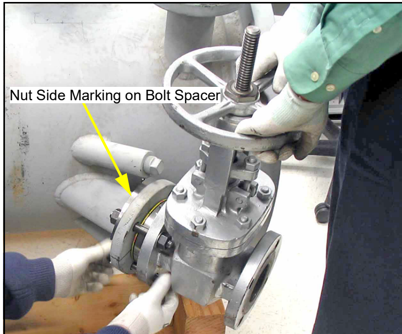
Figure 5: Mounting the Isolation Valve
