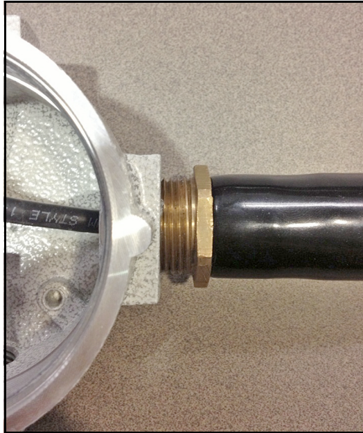
Figure 17: Torquing the Cable Gland
