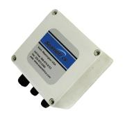
The housing is rugged molded ABS plastic, NEMA 4X rated. It can be wall or panel mounted. The PC42 can be hardwired to the AC main supply or plugged into a standard outlet using the included power cord. Inside there are separate terminals to connect the two devices to the fully isolated supplies.
