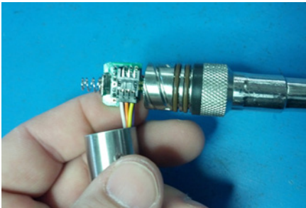
Connector connected properly
