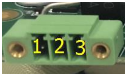
Figure 2.5 Power Socket (DC_IN1)
