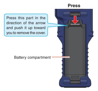
Insert six AA batteries, ensuring that the orientation matches the "+" and "-" marks.
