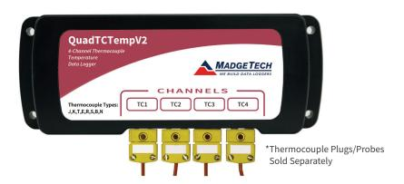
The QuadTCTempV2 is a 4-channel thermocouple data logger with a reading rate of up to 4 Hz. It can measure and record 261,888 readings per channel. To maximize memory capacity, users can enable or disable channels. For easy identification, each channel can be named with up to a ten digit title.
