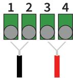
For 2-wire RTD probes, short inputs 3 and 4 together and inputs 1 and 2 together, then connect the RTD lead wires to inputs 2 and 3.
