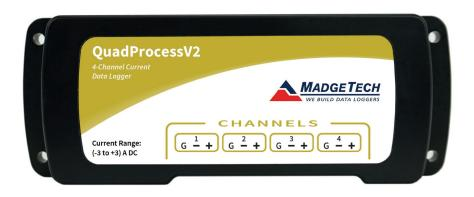
The QuadProcessV2 is an 4-channel, battery powered, low level DC current data logger with a reading rate of up to 4 Hz. It can measure and record 523,776 readings per channel. To maximize memory capacity, users can enable or disable channels. For easy identification, each channel can be named with up to a ten digit title.
