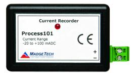
The Process101 is engineered for accuracy and flexibility unequaled in the 4-20mA loop sensor and control industry. It can be inserted almost anywhere because it adds very little resistance to the loop ( $10\Omega$  typical). Since it operates with an internal battery (user replaceable), ground loop errors can be avoided.
