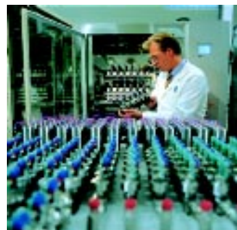
Computerized testing and calibration of pressure transducers.
