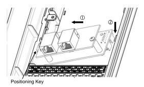
Figure 7: Mounting the Interface Card
