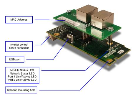
Figure 5: OPC-PRT2 Component Overview (Reverse View)
