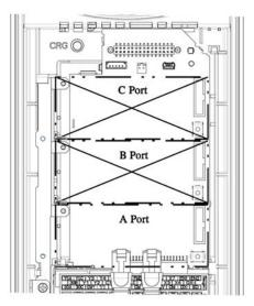
Figure 6: Option Port Locations on 0.4 kW Inverter
