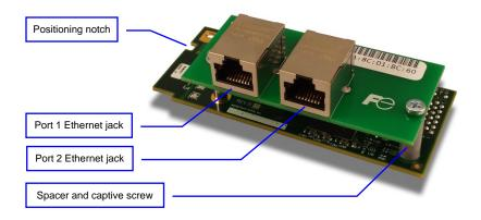
Figure 4: OPC-PRT2 Component Overview (Front View)
