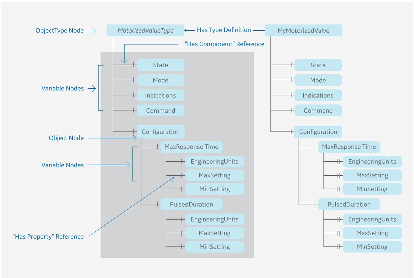
Figure 5 - OPC ObjectType Definition for a Motorized Operated Valve
