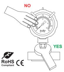
After installation the vent plug can be cut to relieve internal pressure changes in the gauge case that otherwise would have been induced by environmental changes in pressure and/or temperature. Without being vented this change in internal pressure could adversely affect the accuracy of the gauge. If liquid filled, only open vent plugs when the plug is oriented in the vertical position.
