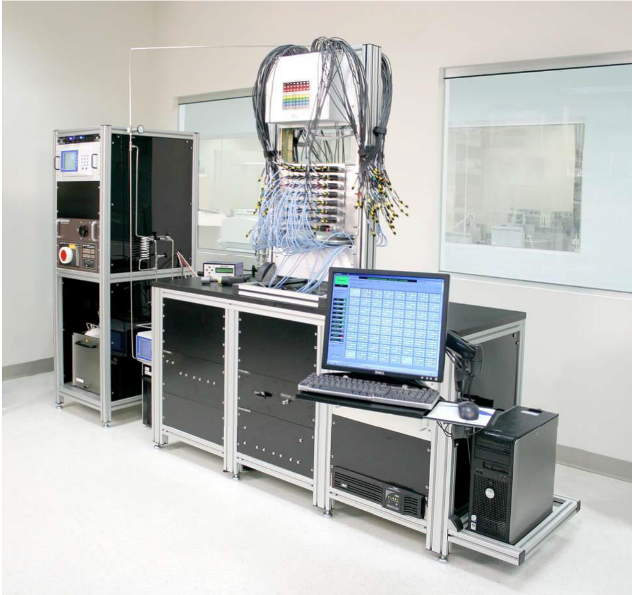
Overall Aluminum Oxide Moisture Probe Calibration System View
