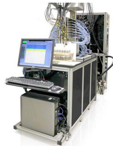
Aluminum Oxide Moisture Probe Calibration System
