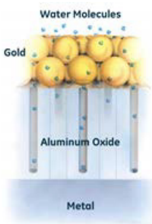
Aluminum Oxide Moisture Sensor Construction
