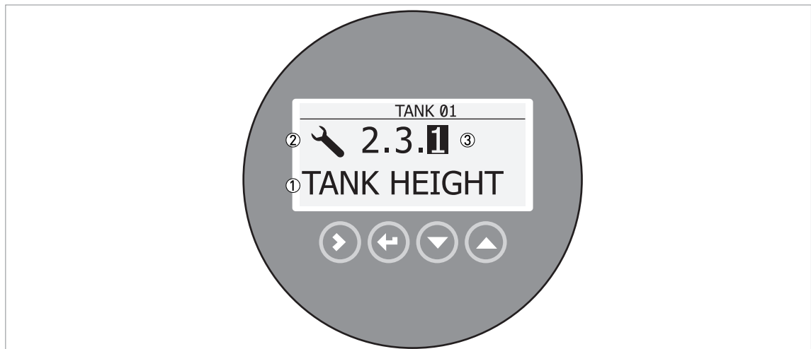
Figure 6-1: Local display screen layout in configuration mode
