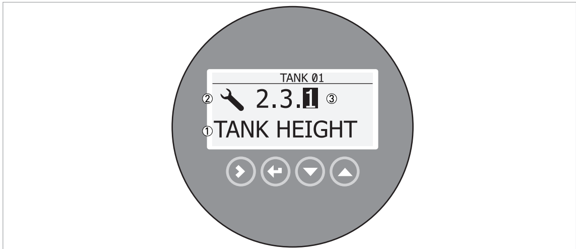
Figure 5-2: Local display screen layout in configuration mode
