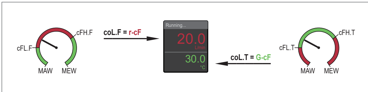
Fig. 20: Colour change. Example: col.F = r-cF ; col.T = G-cF ; current measured values between the limit values.
