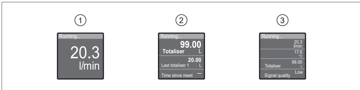
Fig. 6: Switching between the process value displays
