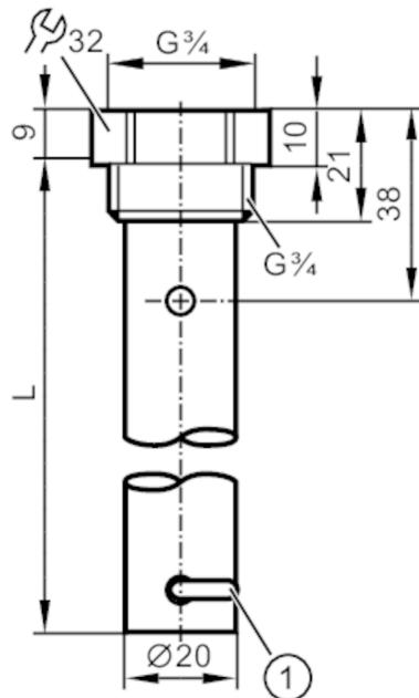
1 Fixing bracket for centring piece
