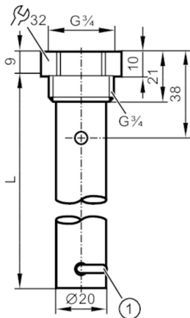
1 Fixing bracket for centring piece
