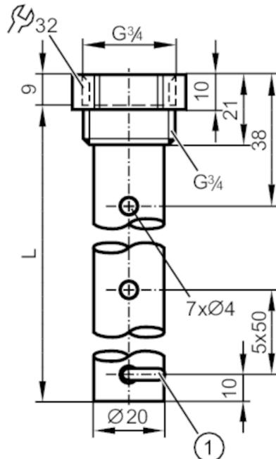
1 fixing bracket for centering piece
