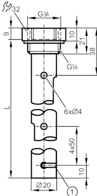
1 fixing bracket for centering piece
