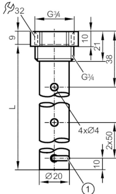
1 fixing bracket for centering piece
