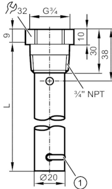
1 fixing bracket for centering piece
