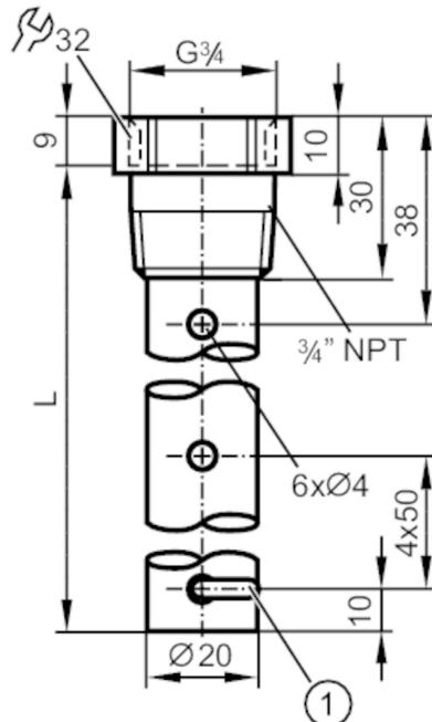
1 fixing bracket for centering piece
