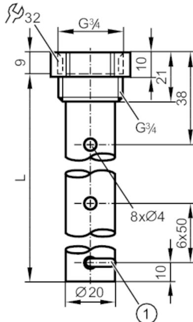
1 fixing bracket for centering piece
