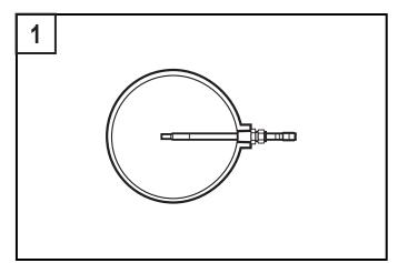
To avoid malfunction a minimum distance between the flow sensor and bends, valves, changes in cross-section or such like must be observed:
