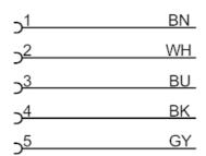
$\begin{array}{ccc} & & & & & & \\ \text{Core colours:} \\ \text{BK =} & & & & \text{black} \\ \text{BN =} & & & \text{brown} \\ \text{BU =} & & & \text{blue} \\ \end{array}$
