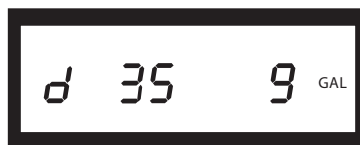
Figure 14: Meter type, digit resolution from the register and unit of measure
