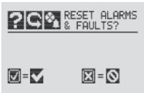
Figure 36. Alarm Reset screen
