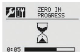
Figure 195. Zero Calibration in Progress
