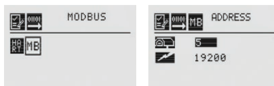
Figure 182. Modbus Configuration Display screen
