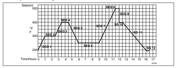
Figure 4-3 Ramp/Soak Profile Example Ramp/Soak Profile Example
