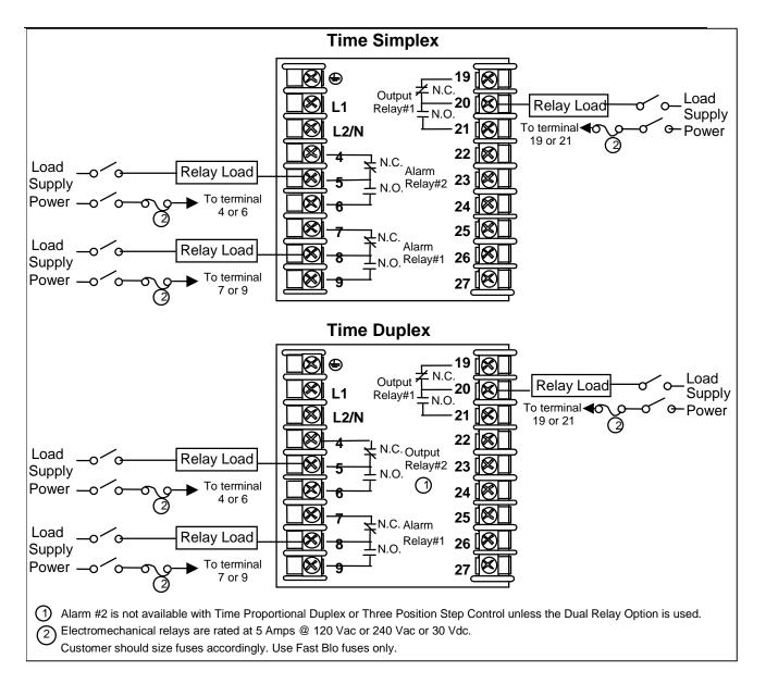
Figure 2-8 Electromechanical Relay Output
