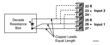
Figure 5-4 Wiring Connections for RTD (Resistance Thermometer Device)
