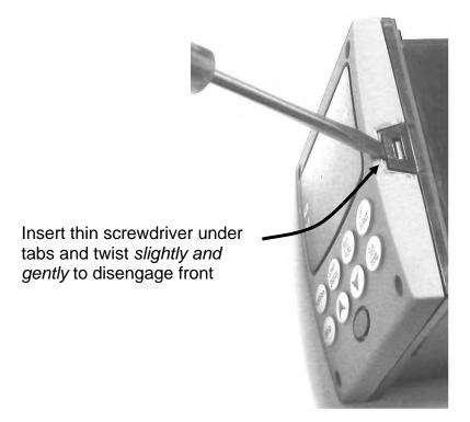
Using a thin screwdriver, *gently* twist the screwdriver to pry the side tabs from the front face. Pry just enough to release it, *otherwise you'll bend or break the tab*. If you break or bend the tab and can't reattach the front snugly, you'll need to reattach the front using the 4 NEMA4 screws provided. See Section 2.5 Mounting.
