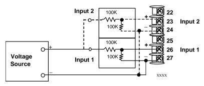
Figure 5-6 Wiring Connections for 0 to 10 Volts
