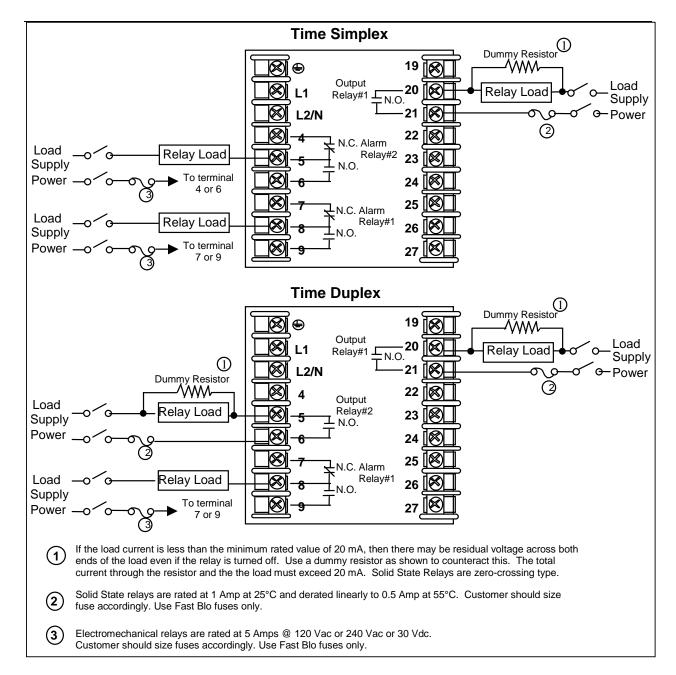
Figure 2-9 Solid State Relay Output
