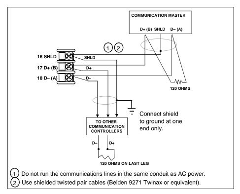
Figure 2-15 RS-422/485 Communications Option Connections
