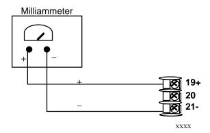
Figure 6-1 Wiring Connections for Calibrating Current Proportional Output
