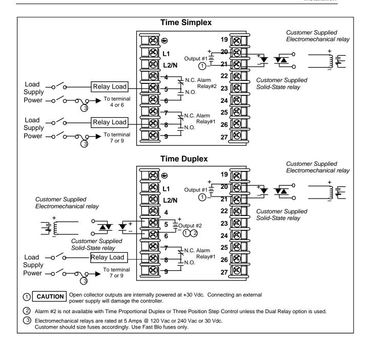
**Figure 2-10 Open Collector Output**
