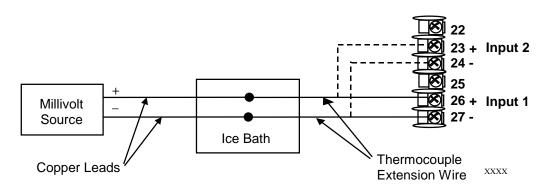
Figure 5-2 Wiring Connections for Thermocouple Inputs Using an Ice Bath
