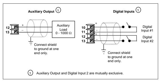
Figure 2-17 Auxiliary Output and Digital Inputs Option Connections
