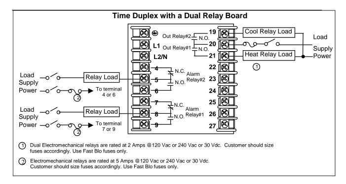
Figure 2-11 Dual Electromechanical Relay Option Output
