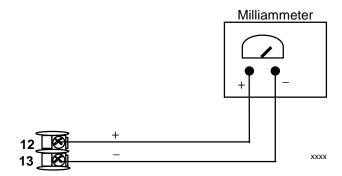
Figure 6-2 Wiring Connections for Calibrating Auxiliary Output
