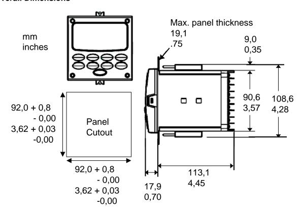
Figure 2-2 Mounting Dimensions (not to scale)
