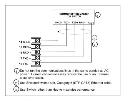
**Figure 2-16 Ethernet Communications Option Connections**
