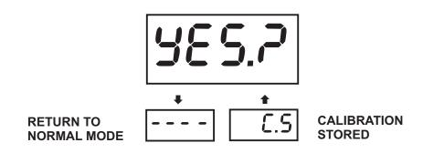
Press **1** to Store calibration (LIT will display **-C.S**-). Calibration is stored in non-volatile memory (even through power interruptions).
