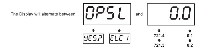
The Output Simulation function controls the digital display 4-20mA output and control relay. Use it to simplify calibration of remote 4-20mA devices such as chart recorders or remote displays, and to test relay set-points.
