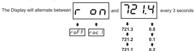
**ROC2** (Level + Echo Loss Alarm) - Relay will be energized when the Relay ON set point is reached.
