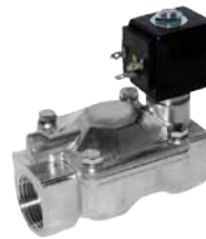
W-P 2-way, N/C Nickel Plated 3/4"-2", 2-230 psi
