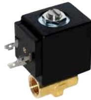
T 2-way, N/C Direct Acting 1/8"-1/4", 0-430 psi
