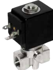
L 2-way, N/C Direct Acting, 316SS 1/8"-1/4", 0-435 psi
