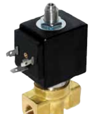
A3 3-way, N/C Direct Acting 1/8"-1/4", 0-290 psi
