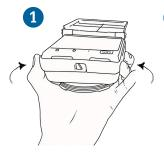
Squeeze both legs to loosen latches
