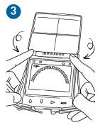
Insert top of cover into transmitter first
