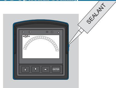
Optional: For a watertight seal (NEMA 4X, IP66 or higher), the Sun Visor must be sealed all around with sealant.
