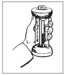
8. Hold FYRITE at 45° angle (Fig. 9) momentarily to allow fluid droplets to drain into the bottom reservoir.
