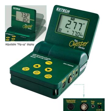
**341350A-P** kit comes with polymer Conductivity cell, glass pH electrode and Thermistor probe
