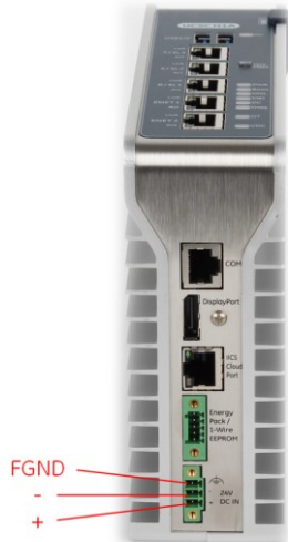
Figure 3: 24 VDC Power Input Connector
