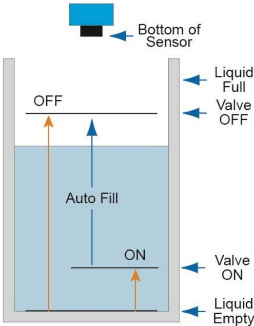
Before starting, take two measurements. 1) Measure the distance from the bottom of the tank to the Valve ON position. 2) Measure the distance from the bottom of the tank to the Valve OFF position. Valve ON will be physically lower than the Valve OFF position.
