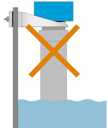
**Note:** The Side Mount Bracket (LM50 series) is not designed for use with stand pipes or as a method to secure stand pipes. There are too few threads to properly hold the sensor and the stand pipe.
