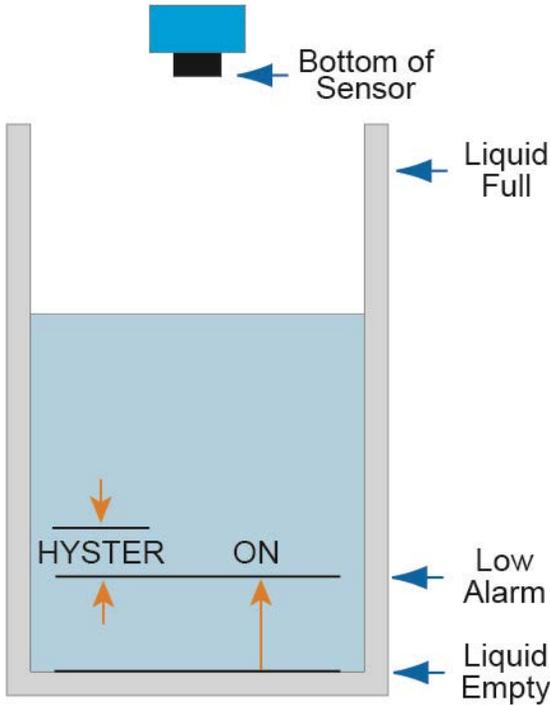
Before starting, measure the distance from the bottom of the tank to the Low Alarm position (ON) in the tank.
