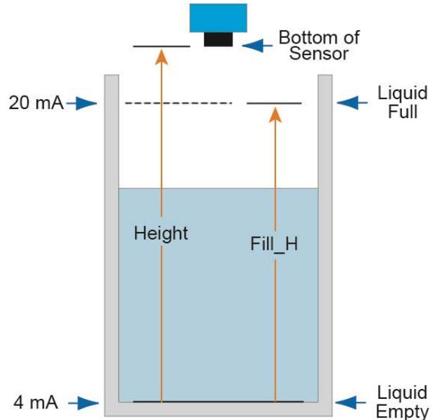
**Note:** The Height and Fill-Height settings also determine the 4 to 20 mA current span. The Height setting determines the 4mA position and the Fill-H setting determines the 20 mA position.
