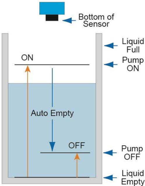
Before starting, take two measurements. 1) Measure the distance from the bottom of the tank to the Pump ON position. 2) Measure the distance from the bottom of the tank to the Pump OFF position. Pump ON will be physically higher than the Pump OFF position.
