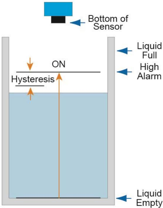
Before starting, measure the distance from the bottom of the tank to the High Alarm position (ON) in the tank.
