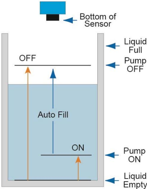
Before starting, take two measurements. 1) Measure the distance from the bottom of the tank to the Pump ON position. 2) Measure the distance from the bottom of the tank to the Pump OFF position. Pump ON will be physically lower than the Pump OFF position.
