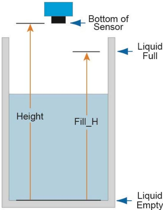
Before starting, take two measurements. 1) Measure the distance from the bottom of the sensor (transducer face) to the bottom of the tank. This will be the HEIGHT setting. 2) Measure the distance from the bottom of the tank to the Maximum Level of Liquid (Full). This will be the FILL-H setting.
