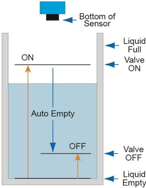
Before starting, take two measurements. 1) Measure the distance from the bottom of the tank to the Valve ON position. 2) Measure the distance from the bottom of the tank to the Valve OFF position. Valve ON will be physically higher than the Valve OFF position.
