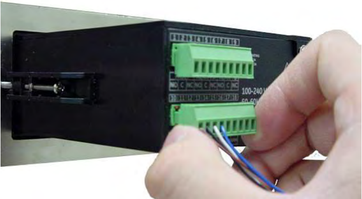
Figure 29: Reinserting the Connector into the Terminal Block
