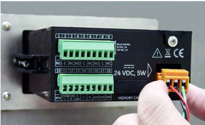
Figure 34: Reinserting the DC Power Connector
