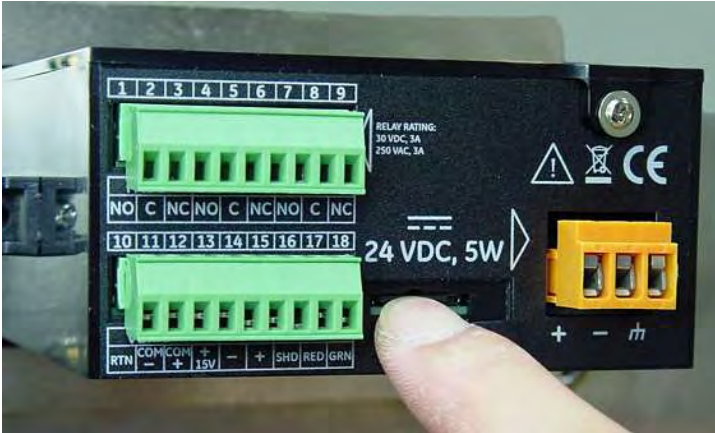
Figure 50: Pushing in on the MicroSD Card
