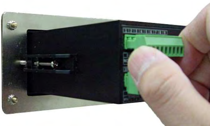
Figure 30: Removing the Upper Connector
