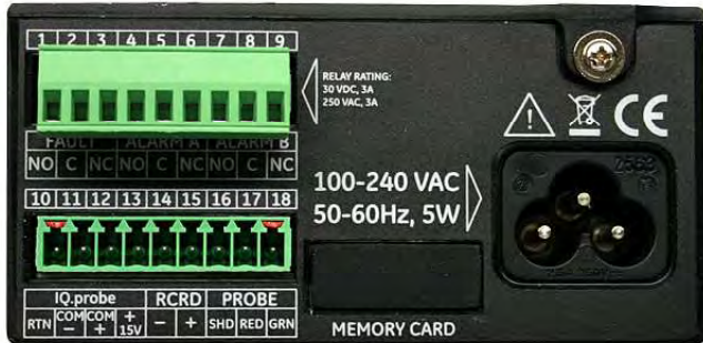
Figure 27: Bottom Connector Removed
