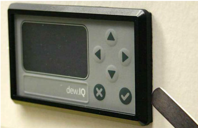
Figure 15: Checking the Gasket Compression
