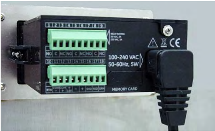
Figure 32: The AC Power Cable Installed
