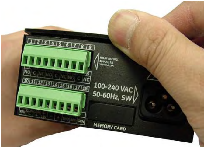
Figure 5: Lifting the Back Edge of the Cover
