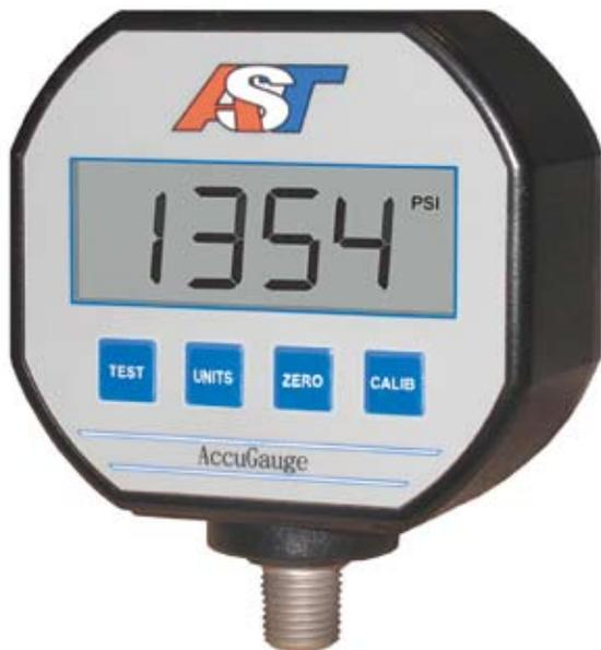
The **AG200** is a media-isolated, digital pressure gauge that offers a 4-20mA output signal with a large LCD display. Utilizing *Krystal Bond™ Technology*, the **AG200** provides the same quality and performance as AST's sensors, with a local readout. The **AG200** also has the option of zero and span calibration, allowing the user to reset the gauge, or adjust the calibration points to their exact needs.
